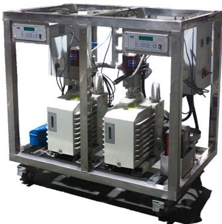
Vacuum Pump for Dynamic Vacuum System
