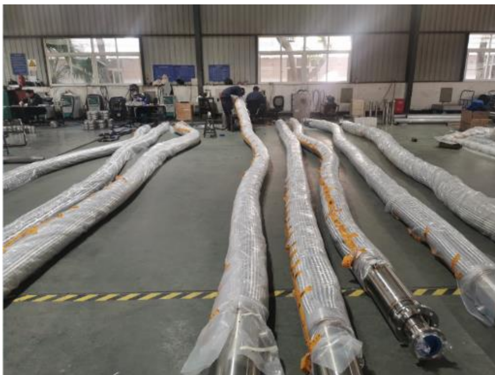
DN150 VI Braided Flexible Hose in manufacturing factory
